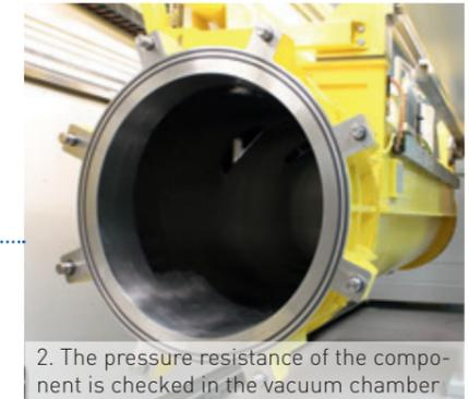
2. The pressure resistance of the component is checked in the vacuum chamber
