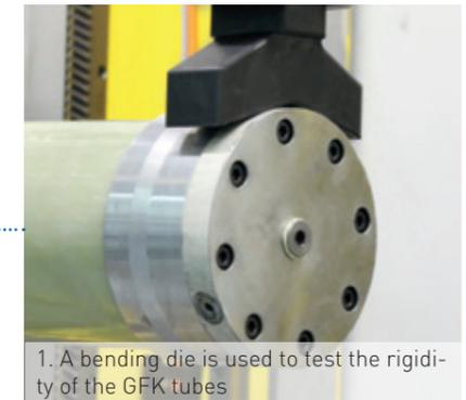
1. A bending die is used to test the rigidity of the GFK tubes
